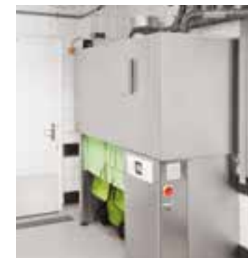
Dehydrated double bin Waste Storage
